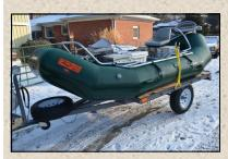
**Standard Trailer, Wheels Under:** This trailer shares the same configuration as the Standard 15' Trailer but has 14" wheels under the deck. The trailer is narrower for narrower garages. Overall width is 82". Total length with boat aboard will be: SF=18'; and SH=19'. The post for the winch is removable so the boat can be moved forward all the way to the ball for storage resulting in 3' to 4' less total length. Deck size 7x8. Price: **\$2,900**
