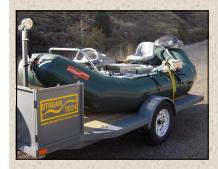
**Cargo Trailer:** Our cargo trailer is built on a 3500 lb axle and measures 99" total outside width and 81" between wheel wells. It includes access walk ways along each side in front and rear of the wheel well. 24" Cargo box front to back and has hinged doors on either side for quick access. Removable winch post Std.. The cargo bay can be modified to accommodate a motorcycle. Length =18.5' Total length with boat aboard will be +3' for SF and +4' for SH. Deck size 7x12. Price: \$ 4,375
