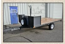
**Cargo Trailer, Wheels Under:** This trailer shares the same configuration as the standard Cargo Trailers but has 14" wheels under the deck. The trailer is narrower at 82". The post for the strap winch is removable to allow moving the boat forward 24" for storage. Length is 18.5'. Deck size 7x12. Price: \$ 4,590
